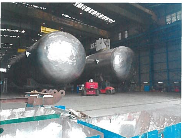
Figure 2. Foam insulated IMO Type C fuel tanks.
